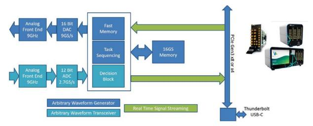
The Proteus architecture in the diagram above provides high-fidelity waveform direct to microwave generation, combined with real-time feedback and high-speed data transfer system. This capability enhances your quantum computing application, while simplifying the design and eliminating many components such as RF signal Generators and Connectorized Components.
